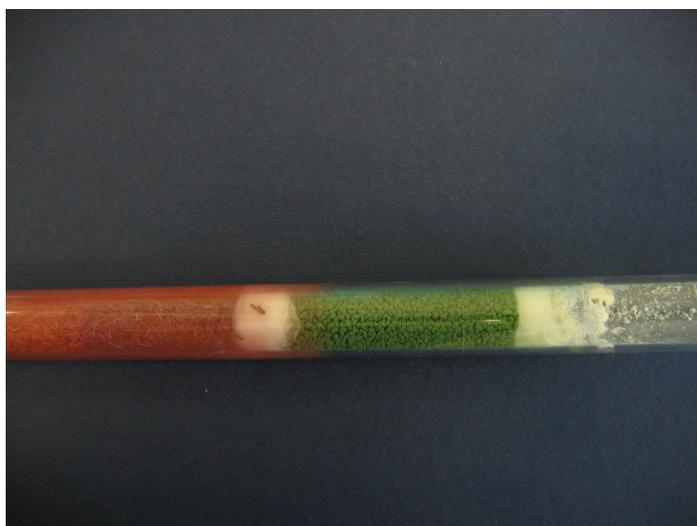
**Fig. 2: Quartz tube with new  $\text{Cr}_2\text{O}_3$  after 40 runs**
