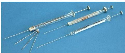
Fig. 54: Syringe and removable needles
