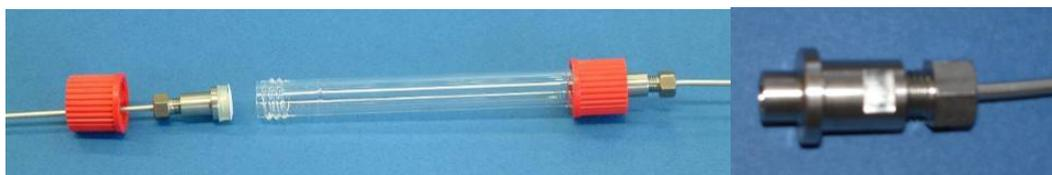
Fig. 21: Water-trap complete with modified filter coupling
