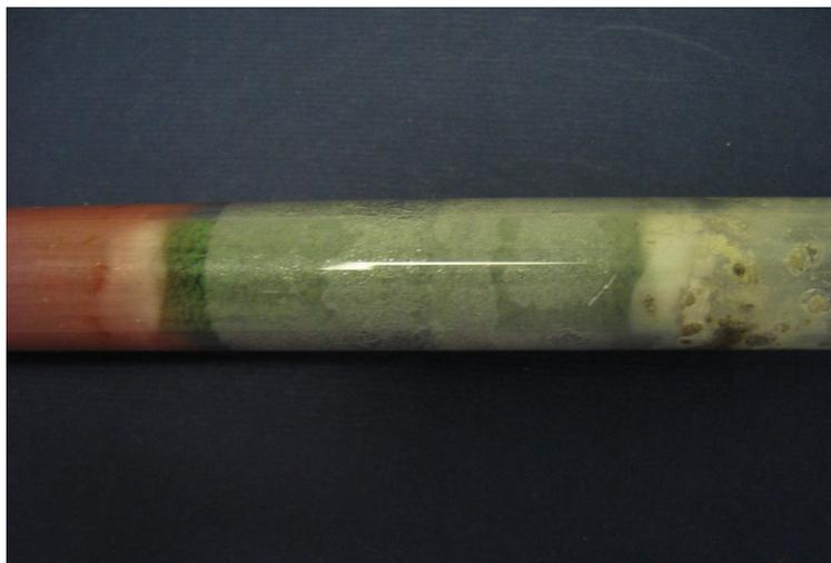
**Fig. 4: Quartz tube with new  $\text{Cr}_2\text{O}_3$  after 250 runs**
