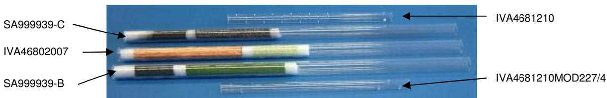
Fig. 14: Prepacked reactors and quartz inserts
